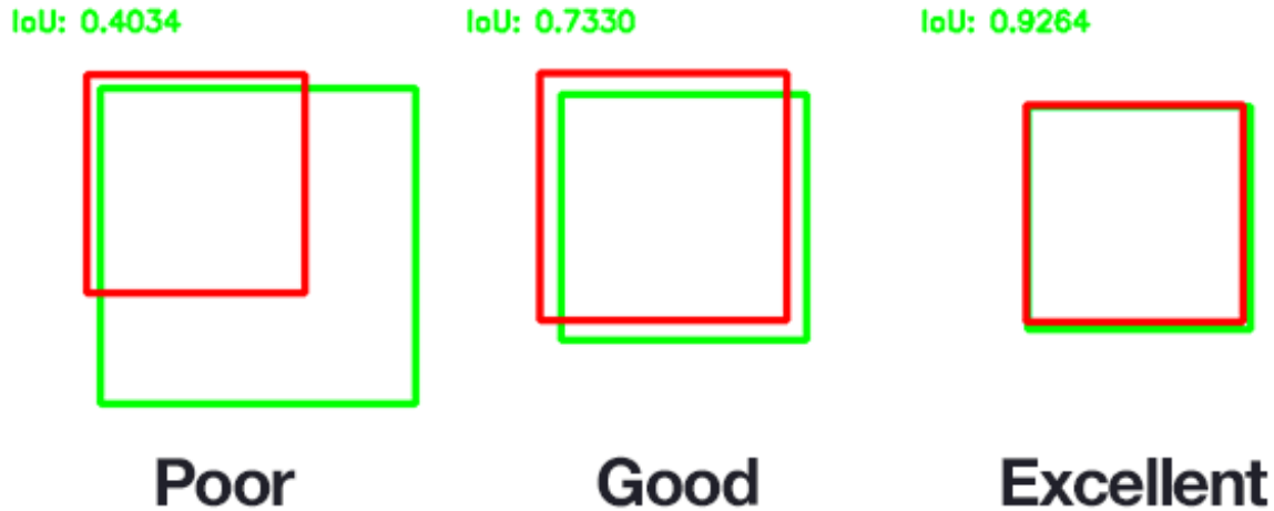
Figure 3.6: Three examples of different IoU values and what type of performance they represent.
